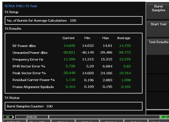
The displayed measurements are colour coded Pass/Fail to either the ETSI published specifications or user defined Test Limits. **Green=Pass, Red=Fail**
